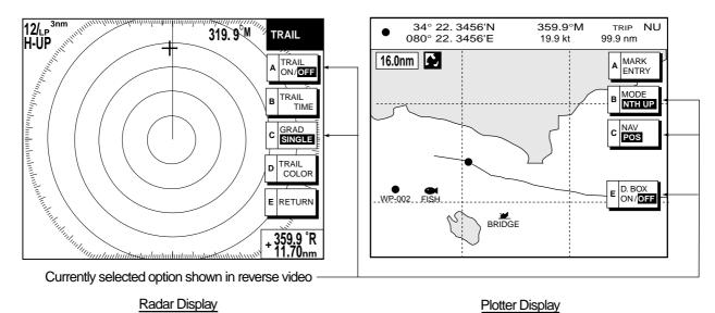
Radar and plotter displays
